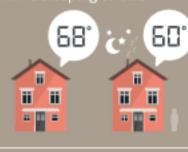
An eight-degree difference in temperature setbacks keeps your HVAC system from working too hard.
